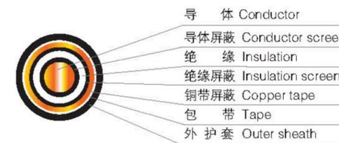
3.6/6kV~26/35kV单芯交联聚乙烯绝缘钢带铠装电力电缆
