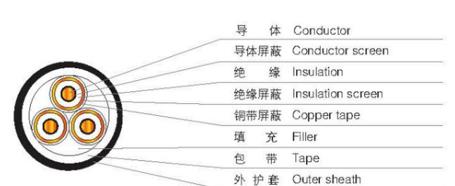
3.6/6kV~26/35kV三芯交联聚乙烯绝缘钢带铠装电力电缆 (YJV22, YJLV22, YJV23, YJLV23)
